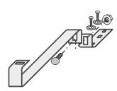
Initially tighten the roof hooks only by hand.
