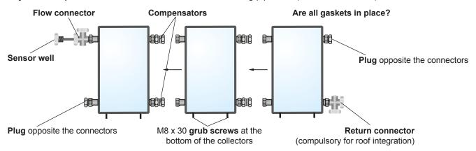
Layout example: 3 F3-1Q collectors, across, single sided connection on the left (max. 5 collectors)
