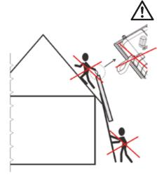
The collector must **not** be pulled onto the roof exclusively by the rivet nuts! Do not step underneath the collector during transport. (see picture)
