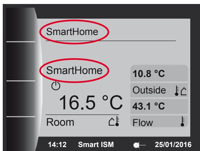
When the components for individual room temperature control are enabled and the SmartHome system's heating control is set up correctly, the heating system or individual heating circuits / heating circuits with mixer are automatically controlled based on demand. This regulates the flow temperature (set temperature) of the circuits according to the heat demand of the rooms. The heat demand is calculated using intelligent algorithms from the SmartHome central unit (wibutler pro).
